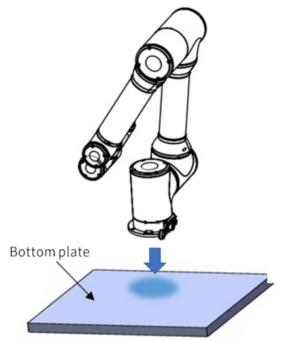
Step1: According to the base size prepare the bottom plate. Step2: Use a foklift to move the robot installation location. Step3: Two or more people slowly lift the robot. According to the installation method to install the robot base installed at the bottom of hole.Install the robot with an Allen Wrench, torque:25N • m.
