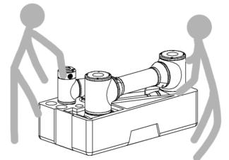
Step :Remove the robot from the foam box and install the robot moving to the installation rack.
