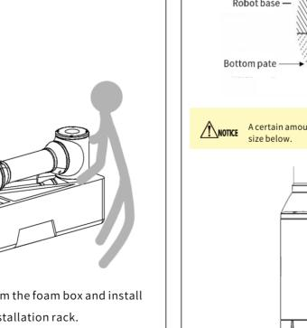
When transporting robots, at least 2 people should support them with their hands and work together. Assist in transporting the robot to the /!\NOTICE installation rack (the entire robot Weight is 21kg).
