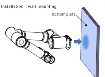
Step1: According to the base size prepare the bottom plate. Step2: Use a foklift to move the robot installation location. Step3: Two or more people slowly lift the robot. According to the installation method to install the robot base installed at the bottom of hole. Install the robot with an Allen Wrench, torque:25N • m.
