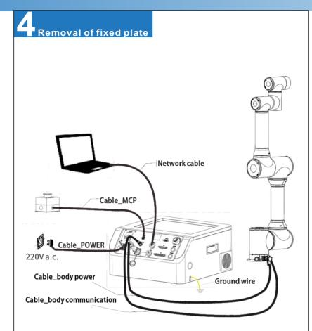
Step1: Install the network cable, ground wire, cable\_MCP, cable\_POWER, cable\_body power and cable\_body communication.
